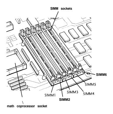
4. Install the SIMMs in the sockets closest to the right side of the main system board first. Position each SIMM so the notch on its edge faces the front of the computer and place it on the left side of the tabs at an angle, as shown below.
